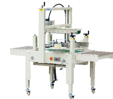
AS423B (Side Sealing Type) Carton Side Sealing Machine 半自动封箱机(泡沫箱款) Power Supply/供给电源: 110V,220-240V/50-60Hz Power/功率: 180W Conveyor Speed/输送速度: 20m/min Max. Carton Size/最大纸箱尺寸: W500xH500mm Min. Carton Size/最小纸箱尺寸: W150xH70mm Width Of Tape/胶带宽度: 50mm or 60mm Machine Size/机器尺寸: 1900x900x1320mm
