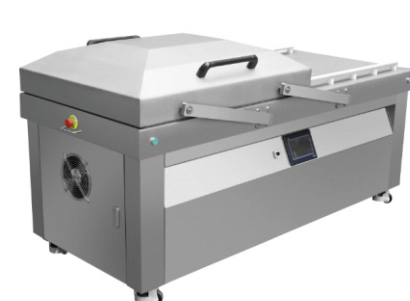
DZP820/2SA & DZP920/2SA Double Chamber Vacuum Packing Machine 双室平板真空包装机 (自动摆盖) Chamber Size/真空室尺寸: 850X800X185mm(DZP820/2SA) 950X880X185mm(DZP920/2SA) Sealing-bar Size/双封条尺寸: 820X10mm(DZP820/2SA) 920X10mm(DZP920/2SA) Distance between sealing bar 封条中心距: 740mm & 800mm Pump Capacity/真空泵: 5KW/200m³ Automatic Cover closing 自动摆盖功能
