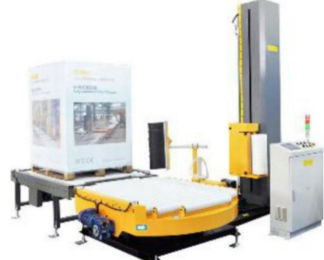
BL2000D(On line model) Pallet Stretch Wrapping Machine 自动缠绕膜包装机(带压顶) Power Supply/电源电压: 220V/50-60Hz 2.9KW Turntable Diameter/转盘直径: Φ2000mm Turntable Height/转盘高度: 500mm Pallet Size/托盘规格: L500-1200×W500-1200×H1800mm Speed of Turntable/转盘转速: 0-15r/min. Max. Loading of Turntable/转盘承载: 2000kgs Percent of Pre-stretch/预拉伸比: 250%
