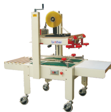
AS223 (Top Sealing Model) Carton Sealing Machine 半自动封箱机 Power Supply/供给电源: 110V,220-240V/50-60Hz Power/功率: 180W Conveyor Speed/输送速度: 20m/min Max. Carton Size/最大纸箱尺寸: W580xH590mm Min. Carton Size/最小纸箱尺寸: W100xH100mm Width Of Tape/胶带宽度: 50mm or 60mm Machine Size/机器尺寸: 1545x815x1475mm
