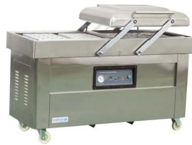
DZ400/2SB & DZ500/2SB & DZ600/2SB Double Chamber Vacuum Packing Machine 双室真空包装机 Chamber Size/真空室尺寸: 540X470X50mm(DZ400/2SB) 540X570X50mm(DZ500/2SB) 540X670X50mm(DZ600/2SB) Sealing-bar Size/双封条尺寸: 400X10mm(DZ400/2SB) 500X10mm(DZ500/2SB) & 600X10mm(DZ600/2SB) Pump Capacity/真空泵: 900W / 20m³ (DZ400/2SB) 2PCS 20m³ for DZ500/2SB & 1.5KW/40m³ for DZ600/2SB Options: Nitrogen Filling Function 可选充氮气功能
