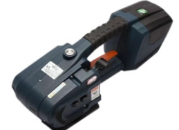
JDC13 & JDC16 Battery Strapping Tool 电动打包机 Strap Type/适用打包带: PP/PET Strap Width/带宽: 13mm or 16mm Lithium Battery/锂电池: 4.0Ah Max. Tension: Up to 280kg
