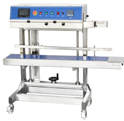
FPM600L/S Vertical Band Sealer With Ink-jet Printer 重载立式喷码封口机 Sealing Width/封口宽度: 10mm Conveyor Width/输送台宽度: 200mm Conveyor Loading/输送台载重: 15kgs Max. Distance from C.V to Sealing: 600mm Printer Specification same as FPM200W
