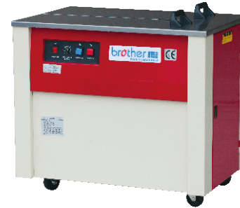
KZB-I Semi-auto Strapping Machine 半自动捆扎机 Power Supply/电源电压: 110V, 220V/50-60Hz Strapping Tension/捆扎力: 40-400N Adjustable Strapping Speed/捆扎速度: 1.5 sec./cycle Strap Width/适用机用带宽度: 9-15mm
