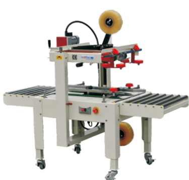
FXJ5050II Carton Sealing Machine 半自动封箱机 Power Supply/供给电源: 110V,220-240V/50-60Hz Power/功率: 180W Conveyor Speed/输送速度: 20m/min Max. Carton Size/最大纸箱尺寸: W500xH500mm Min. Carton Size/最小纸箱尺寸: W100xH100mm Width Of Tape/胶带宽度: 50mm or 60mm Machine Size/机器尺寸: 1630x800x1230mm
