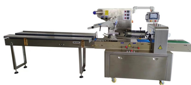
DZB600/SV Automatic Pillow Packing Machine 自动枕式包装机 Power Supply/电源: 110V or 220-240V/50-60Hz 3.2KW Packing Capacity/包装速度: 10-60 bags/min. Bag Size/制袋尺寸: L150-500mm, W20-280mm, H5-110mm Max. Film Width/最大膜宽: 600mm 3 Servo Motors Model/三伺服
