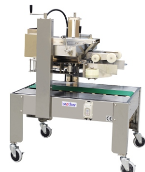
AS623 (Suit for Bubble Box) Carton Side Sealing Machine 半自动封箱机(水产泡沫箱款) Power Supply/供给电源: 110V,220-240V/50-60Hz Power/功率: 240W Conveyor Speed/输送速度: 20m/min Max. Carton Size/最大纸箱尺寸: W500xH430mm Min. Carton Size/最小纸箱尺寸: W280xH100mm Width Of Tape/胶带宽度: 50mm or 60mm Machine Size/机器尺寸: 1000x900x1350mm
