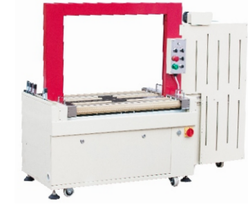
APM8060C (Online Model) Automatic Strapping Machine 在线式自动捆扎机 Power Supply/电源电压: 3P, 220V or 380V/50-60Hz Strapping Tension/捆扎力: 40-600N Adjustable Strapping Speed/捆扎速度: 2.18sec./cycle Strap Width/适用机用带宽度: 9-15mm Arch Size/框架尺寸: W800XH600mm Working Table Height/工作台面高度: 650mm
