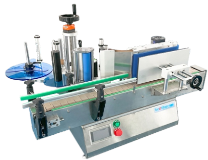
TRLB120B Tabletop Round Bottle Labeling Machine 台式圆瓶贴标机 (直线式) Suitable Bottle Diameter/瓶子直径: 25-100mm Bottle Height/瓶子高度: 25mm-230mm Label Size/标签尺寸: L20-320mm W15-175mm Labeling Speed/贴标速度: 30-80 bottles/min.
