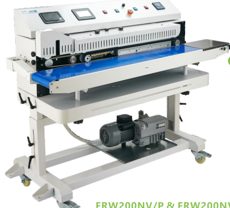
FRW200NV/P & FRW200NV/S Vacuum & Nitrogen Filling Band Sealer 真空&充气喷码封口机 (平移款) Vacuum Pump Capacity/真空泵: 900W/20m³ Printing Font Height/字体高度: 1.5-12.7mm Max. Printing Lines/最大印字行数: 6 lines Ink Color/墨盒颜色: Black/Red/Green/Blue/White Languages/操作语言: 中文/English/Arabic/Korea Portuguese/Spanish/Japanese/Turkish/Thai Vacuum Function Operate during the translation process.
