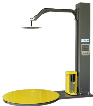
BL2000B(With Top press) Pallet Stretch Wrapping Machine 自动缠绕膜包装机(带压顶) Power Supply/电源电压: 220V/50-60Hz Turntable Diameter/转盘直径: Φ1650mm (Φ2000mm are option) Truntable Thickness/装盘厚度: 85mm Speed of Turntable/转盘转速: 0-12r/min. Max. Wrapper Height/包装高度: 2000mm Max. Loading of Turntable/转盘承载: 2000kgs Percent of Pre-stretch/预拉伸比: 250%
