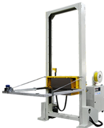
APH105A Automatic Pallet Horizontal Strapping Machine 自动水平式捆扎机 Power Supply/电源电压: 3P, 220V or 380V/50-60Hz Strapping Speed/捆扎速度: 15 sec./cycle Strapping Tension/捆扎力: 10-90kg Adjustable Strap Width/适用机用带宽度: 9-15mm Arch Size/轨道尺寸: L1500XW1500mm
