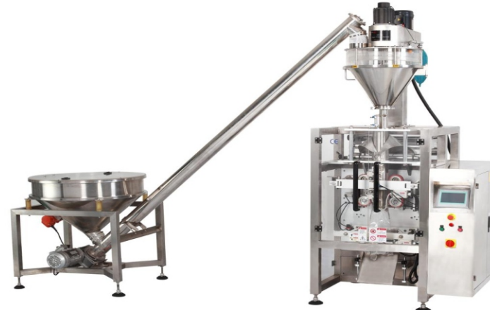
BVP420F (Powder Type) Automatic Vertical Packing Machine 自动立式包装机 Packing Capacity/包装容量: 150-1000ml Bag Size/制袋尺寸: L80-300, W50-200mm Shape of bag/制袋形式: 3 side sealing, 4side sealing & back side sealing are option
