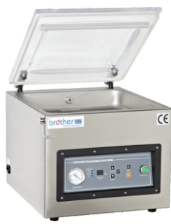
VM400TE/A & VM400TE/B & VM400TE/C Tabletop Vacuum Packaging Machine 台式真空包装机 Chamber Size/真空室尺寸: 440X420X75mm Sealing-bar Size/热封条尺寸: 400X10mm VM400TE/A(Single bar) & VM400TE/B(Double bar) Pump Capacity/真空泵: 900W / 20m³ Vacuum Time/真空循环时间: 10-25 sec. Options: Nitrogen Filling Function 可选充氮气功能
