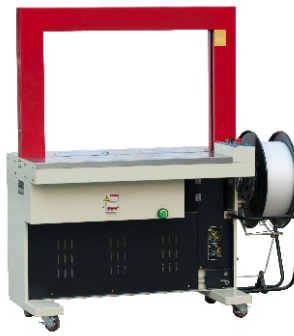
WG22XN (PCB Model) Automatic Strapping Machine 全自动捆扎机 Power Supply/电源电压: 3P, 220V or 380V/50-60Hz Strapping Tension/捆扎力: 100-500N Adjustable Strapping Speed/捆扎速度: 2.5 sec./cycle Strap Width/适用机用带宽度: 9-15mm Arch Size/框架尺寸: W800XH600mm
