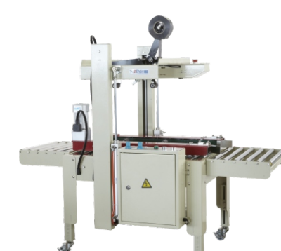
AS823A (Random Model) Carton Sealing Machine for Random size box 半自动封箱机(自动尺寸调节款) Power Supply/供给电源: 110V,220-240V/50-60Hz Power/功率: 240W Conveyor Speed/输送速度: 20m/min Max. Carton Size/最大纸箱尺寸: W500xH500mm Min. Carton Size/最小纸箱尺寸: W150xH120mm Width Of Tape/胶带宽度: 50mm or 60mm Air Source/气源: 0.4~0.8Mpa & 450l/min.
