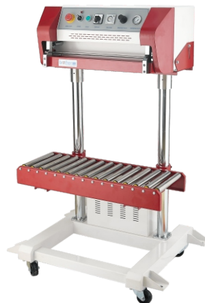
QF600L & QF600L/S Vertical Pneumatic Sealing Machine 气动大袋立式封口机 Sealing Width/封口宽度: 10mm Sealing Length/封口长度: 600mm Distance from table to sealing: 150-800mm Max. Roller table Loading: 50kg Sealing Header angle adjustable 20degree Options: * Double Sealing * 700/800/1000mm Sealing Length.
