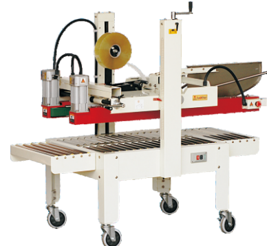
AS323 (Auto. Flap-folding Model) Carton Sealing Machine 半自动封箱机 Power Supply/供给电源: 110V,220-240V/50-60Hz Power/功率: 180W Conveyor Speed/输送速度: 20m/min Max. Carton Size/最大纸箱尺寸: L600xW450xH600mm Min. Carton Size/最小纸箱尺寸: L150xW160xH100mm Width Of Tape/胶带宽度: 50mm or 60mm Machine Size/机器尺寸: 1910x870x1535mm
