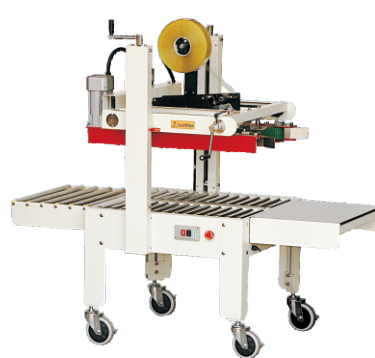
AS123 (Top Sealing Model) Carton Sealing Machine 半自动封箱机 Power Supply/供给电源: 110V,220-240V/50-60Hz Power/功率: 180W Conveyor Speed/输送速度: 20m/min Max. Carton Size/最大纸箱尺寸: W500xH600mm Min. Carton Size/最小纸箱尺寸: W100xH100mm Width Of Tape/胶带宽度: 50mm or 60mm Machine Size/机器尺寸: 1545x815x1475mm
