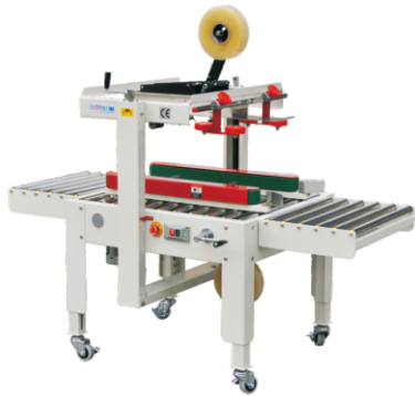
FXJ5050I Carton Sealing Machine 半自动封箱机 Power Supply/供给电源: 110V,220-240V/50-60Hz Power/功率: 180W Conveyor Speed/输送速度: 20m/min Max. Carton Size/最大纸箱尺寸: W500xH500mm Min. Carton Size/最小纸箱尺寸: W100xH100mm Width Of Tape/胶带宽度: 50mm or 60mm Machine Size/机器尺寸: 1660x850x1260mm Option: 3inch tape & overlap (Model FXJ5050/31)
