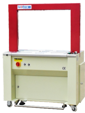
AP8060/PC (PCB Model) Automatic Strapping Machine 全自动捆扎机 Power Supply/电源电压: 110V or 220-240V/50-60Hz Strapping Tension/捆扎力: 40-600N Adjustable Strapping Speed/捆扎速度: 2.2sec./cycle Strap Width/适用机用带宽度: 9-15mm Arch Size/框架尺寸: W800XH600mm
