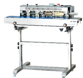
FRD1000LD/P & FRD1000LD/S Solid-Ink Coding Band Sealer 墨轮印字连续封口机 (带落地脚架) Sealing Width/封口宽度: 10mm Sealing Speed/封口速度: 0-24m/min. Conveyor Width/输送台宽度: 150mm Printing letter/印字数: 2 lines 15 letters
