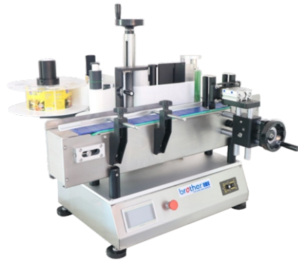
TRLB120A Tabletop Round Bottle Labeling Machine 台式圆瓶贴标机 (抱瓶式) Suitable Bottle Diameter/瓶子直径: 25-100mm Bottle Height/瓶子高度: 25mm-300mm Label Size/标签尺寸: L20-285mm W20-175mm Labeling Speed/贴标速度: 15-50 bottles/min.
