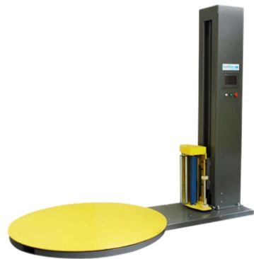
BL2000A & BL2000P Pallet Stretch Wrapping Machine 自动缠绕膜包装机 Power Supply/电源电压: 3P,220V or 380V/50-60Hz Turntable Diameter/转盘直径: Φ1650mm (Φ2000mm are option) Truntable Thickness/装盘厚度: 85mm Speed of Turntable/转盘转速: 0-12r/min. Max. Wrapper Height/包装高度: 2000mm Max. Loading of Turntable/转盘承载: 2000kgs Percent of Pre-stretch/预拉伸比: 250% (BL2000P)
