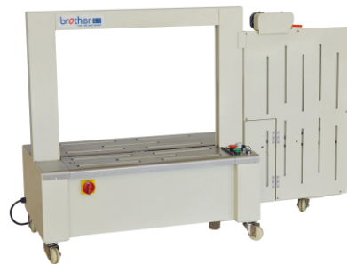
APM8060 (Low Table Model) Automatic Strapping Machine 全自动捆扎机 Power Supply/电源电压: 3P, 220V or 380V/50-60Hz Strapping Tension/捆扎力: 40-600N Adjustable Strapping Speed/捆扎速度: 2.18sec./cycle Strap Width/适用机用带宽度: 9-15mm Arch Size/框架尺寸: W800XH600mm Working Table Height/工作台面高度: 650mm
