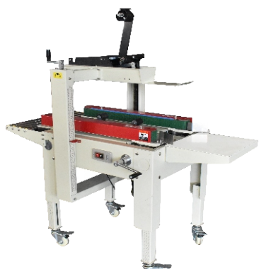
FXJ4030X Carton Sealing Machine for E-commerce Box 半自动封箱机(电商款) Power Supply/供给电源: 110V,220-240V/50-60Hz Power/功率: 80W Conveyor Speed/输送速度: 20m/min Max. Carton Size/最大纸箱尺寸: W300xH400mm Min. Carton Size/最小纸箱尺寸: W80xH90mm Width Of Tape/胶带宽度: 48mm or 50mm
