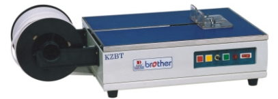
KZBT Tabletop Strapping Machine 台式捆扎机 Strapping Tension/捆扎力: 40-100N Adjustable Strapping Speed/捆扎速度: 5 sec./cycle Strap Width/适用机用带宽度: 6-12mm
