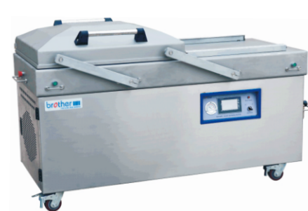
DZP680/2SA & DZP850/2SA Double Chamber Vacuum Packing Machine 双室平板真空包装机 (自动摆盖) Chamber Size/真空室尺寸: 700X550X150mm(DZP680/2SA) 880X600X150mm(DZP850/2SA) Sealing-bar Size/双封条尺寸: 680X10mm(DZP680/2SA) 850X10mm(DZP850/2SA) Distance between sealing bar 封条中心距: 500mm & 540mm Pump Capacity/真空泵: 3KW/100m³ (DZP680/2SA) 5KW/200m³ (DZP850/2SA) Automatic Cover closing 自动摆盖功能
