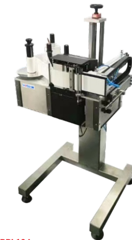
BPL104 Online Printing & Labeling Machine 即时打印贴标机 Suitable Product Height: 5-300mm Label Size: L30-200mm W30-110mm
