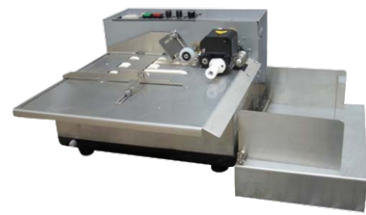
MY380F/W Solid-ink Coding Machine 固体墨轮标示机 Max. Printing Line/最多印字符数: 11 lines 10letters(T type letter) 8 lines 8letters ( R type letter) Max. Object Size/最大印物尺寸: L45-500mm W30-300mm
