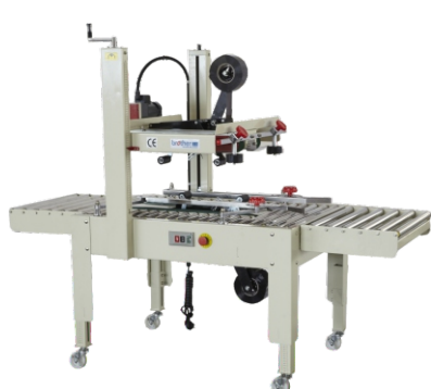
FXJ6060 / FXJ8060 Carton Sealing Machine 半自动封箱机 Power Supply/供给电源: 110V,220-240V/50-60Hz Power/功率: 240W Max. Carton Size/最大纸箱尺寸: W600xH600mm (FXJ6060) Max. Carton Size/最大纸箱尺寸: W600xH800mm (FXJ8060) Min. Carton Size/最小纸箱尺寸: W150xH120mm Width Of Tape/胶带宽度: 50mm or 60mm or 75mm
