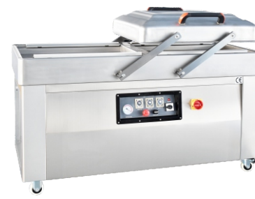
DZ400/2SR & DZ500/2SR & DZ600/2SR Double Chamber Vacuum Packing Machine 双室真空包装机 Chamber Size/真空室尺寸: 540X470X50mm(DZ400/2SR) 540X570X50mm(DZ500/2SR) 540X670X50mm(DZ600/2SR) Sealing-bar Size/双封条尺寸: 400X10mm(DZ400/2SR) 500X10mm(DZ500/2SB) & 600X10mm(DZ600/2SB) Pump Capacity/真空泵: 900W / 20m³ (DZ400/2SB) 2PCS 20m³ for DZ500/2SB & 1.5KW/40m³ for DZ600/2SB Options: Nitrogen Filling Function 可选充氮气功能
