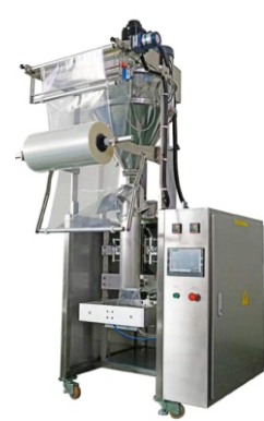
BVP-80IIF Automatic Powder Packing Machine 自动粉末包装机 Packing Capacity/包装容量: 100g-1kg Bag Size/制袋尺寸: L60-300mm, W40-200mm Packing Speed/包装速度: 10-30bags/min. Shape of bag/制袋形式: Back Sealing, Three Side Sealing & Four side Sealing are option.
