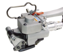
XQD-19E & XDQ-25E Pneumatic Strapping Machine 气动打包机 Strap Width: 13-19mm or 20-25mm Max. Strapping Tension: 3500N Air Source/气压: 0.5-0.8Mpa
