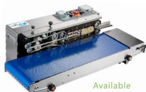
FRD1000W/S250 Solid-Ink Coding Band Sealer 墨轮印字连续封口机 (加宽输送台) Sealing Width/封口宽度: 10mm Sealing Speed/封口速度: 0-24m/min. Conveyor Width/输送台宽度: 250mm Printing letter/印字数: 2 lines 15 letters
