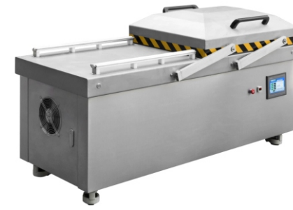
DZP620/2SA & DZP720/2SA Double Chamber Vacuum Packing Machine 双室平板真空包装机 (自动摆盖) Chamber Size/真空室尺寸: 650X550X150mm(DZP620/2SA) 750X600X150mm(DZP720/2SA) Sealing-bar Size/双封条尺寸: 620X10mm(DZP620/2SA) 720X10mm(DZP720/2SA) Distance between sealing bar 封条中心距: 500mm & 540mm Pump Capacity/真空泵: 2.2KW/63m³ (DZP620/2SA) 3KW/100m³ (DZP720/2SA) Automatic Cover closing 自动摆盖功能
