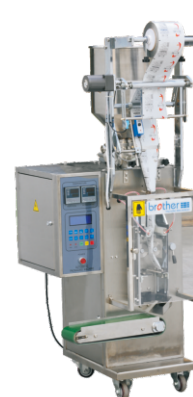
DXDL80C (Liquid Type) Automatic Vertical Packing Machine 自动立式包装机 Packing Capacity/包装容量: 10-100ml Bag Size/制袋尺寸: L40-150, W30-100mm Shape of bag/制袋形式: 3 side sealing, 4side sealing & back side sealing are option
