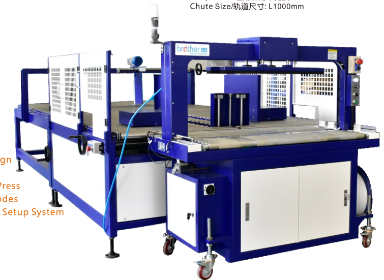
BRO-305RP High Speed Corrugated Strapper With Integrated Squaring System 高速瓦楞箱捆扎机 (带自动整齐理料输送线) Power Supply/电源电压: 3Phase, 220V/60Hz or 380V/50-60Hz 2.4KW Strapping Speed/捆扎速度: Up to 25bundles/min. PP Strap Size/捆扎带规格: W5mm or 6mm, T0.5-0.8mm Arch Size/龙门架尺寸: W1250*H500mm Min. bundle Size: L250*W200*H60mm Working Table Height: 850mm Air Source: 0.4-0.6Mpa
