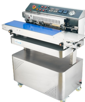
FRV1000N/P & FRV1000N/S Vacuum & Nitrogen Filling Band Sealer 真空&充气封口机 (With Ink Coding) Sealing Width/封口宽度: 10mm Sealing Speed/封口速度: 0-24m/min. Pump Capacity/真空泵: 900W/20m³ Air source: 1-2bar Available Vacuum Seal only or Nitrogen Filling only or Vacuum & Nitrogen filling both. 可选真空封口或单充气封口或同时。
