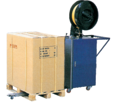
DBA130A Semi-auto. Pallet Strapping Machine 半自动栈板捆扎机 Power Supply/电源电压: 3P, 220V or 380V/50-60Hz Strapping Speed/捆扎速度: 2.5 sec./cycle Strapping Tension/捆扎力: 40-600N Adjustable Strap Width/适用机用带宽度: 9-15mm Chute Size/轨道尺寸: L1000mm
