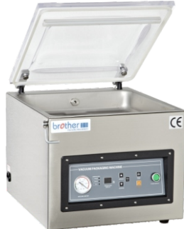
VM500TE/A & VM500TE/B Tabletop Vacuum Packaging Machine 台式真空包装机 Chamber Size/真空室尺寸: 525X525X100mm Sealing-bar Size/热封条尺寸: 500X10mm VM500TE/A(Single bar) & VM500TE/B(Double bar) Pump Capacity/真空泵: 900W / 20m³ Vacuum Time/真空循环时间: 15-30 sec. Options: Nitrogen Filling Function 可选充氮气功能
