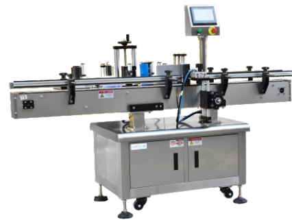
ARLB160A Automatic Labeling Machine 自动圆瓶贴标机 (抱瓶式) Suitable Bottle Diameter/瓶子直径: 30-120mm Label Size/标签尺寸: L30-180mm W30-130mm Labeling Speed/贴标速度: 10-40 bottles/min. Online Model ARLB160B, speed up to 60bpm. Other Diameter bottle available.
