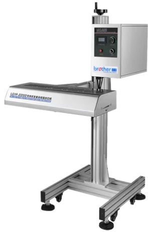
LGYF2200 Online Continuous Induction Sealer 在线式感应封口机 Power Supply/电源: 110V or 220V/50-60Hz, 2.3KW Sealing Diameter/封口直径: Φ30-150mm Vertical Adjusting Height/垂直可调范围: 0-800mm Horizontal Adjusting Size/横向可调范围: 0-260mm Sealing Speed/速度: 80-300pcs/min Stainless Steel & Aluminum Body
