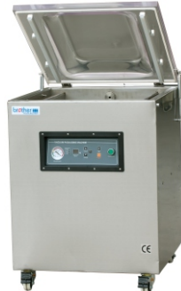
VM600E/A & VM600E/B Vacuum Packaging Machine 真空包装机 Chamber Size/真空室尺寸: 625X625X100mm Sealing-bar Size/热封条尺寸: 600X10mm VM600E/A(Single bar) & VM600E/B(Double bar) Pump Capacity/真空泵: 1.5KW / 40m³ Vacuum Time/真空循环时间: 10-20 sec. Options: Nitrogen Filling Function 可选充氮气功能
