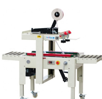
FXJ4030D Carton Sealing Machine for E-commerce Box 半自动封箱机(电商款) Power Supply/供给电源: 110V,220-240V/50-60Hz Power/功率: 120W Conveyor Speed/输送速度: 20m/min Max. Carton Size/最大纸箱尺寸: W300xH400mm Min. Carton Size/最小纸箱尺寸: W80xH40mm Width Of Tape/胶带宽度: 48mm or 50mm
