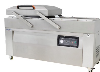
DZ700/2SB & DZ800/2SB Double Chamber Vacuum Packing Machine 双室平板真空包装机 Chamber Size/真空室尺寸: 700X500X90mm (DZ700/2SB) 830X750X90mm (DZ800/2SB) Sealing-bar Size/双封条尺寸: 700X10mm (DZ700/2SB) 800X10mm (DZ800/2SB) Distance between sealing bar 封条中心距: 540mm & 600mm Pump Capacity/真空泵: 2KW/63m³ (DZ700/2SB) 3KW/100m³ (DZ800/2SB) Options: Nitrogen Filling Function 可选充氮气功能
