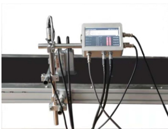
MX1 Inline Ink-jet Printer 在线式喷码机 Printing Font Height/字体高度: 1.5-12.7mm Max. Printing Lines/最大喷码行数: 6 lines Languages/操作语言: 中文, English, Arabic, Turkish, Spanish, Portuguese, Korean, Russian
