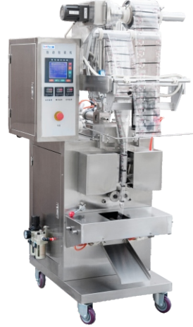
DXDL-S100 Automatic Liquid Packing Machine 自动液体包装机 Filling Capacity/灌装容量: 5-100ml Bag Size/制袋尺寸: L50-150mm, W25-120mm Film Width/卷膜宽度: W60-240mm Packing Speed/包装速度: 30-60bag/min. Air Source/气源: 0.7Mpa 450nl/min.
