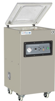
VM400E/A & VM400E/B Vacuum Packaging Machine 真空包装机 Chamber Size/真空室尺寸: 440X420X75mm Sealing-bar Size/热封条尺寸: 400X10mm VM400E/A(Single bar) & VM400E/B(Double bar) Pump Capacity/真空泵: 900W / 20m³ Vacuum Time/真空循环时间: 10-25 sec. Options: Nitrogen Filling Function 可选充氮气功能
