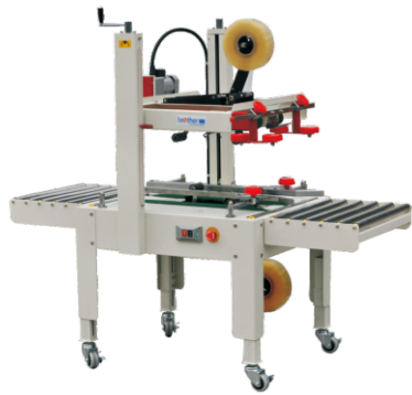
FXJ6050 Carton Sealing Machine 半自动封箱机 Power Supply/供给电源: 110V,220-240V/50-60Hz Power/功率: 180W Conveyor Speed/输送速度: 20m/min Max. Carton Size/最大纸箱尺寸: W500xH600mm Min. Carton Size/最小纸箱尺寸: W150xH120mm Width Of Tape/胶带宽度: 50mm or 60mm Machine Size/机器尺寸: 1630x800x1330mm Option: 3inch tape & overlap (Model FXJ6050/31)
