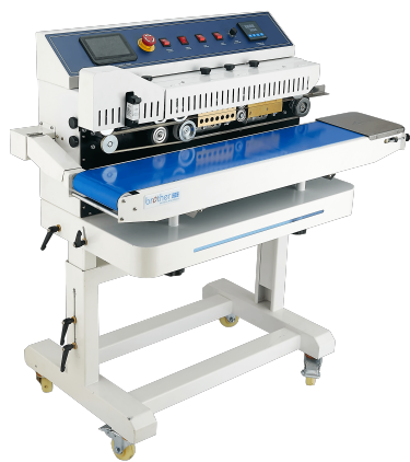
FPM200W (With Ink-jet Printer) Heavy Duty Band Sealer (New) 重载喷码封口机 Sealing Width/封口宽度: 10mm Printing Font Height/字体高度: 1.5-12.7mm Max. Printing Lines/最大印字行数: 6 lines Ink Color/墨盒颜色: Black/Red/Green/Blue/White Languages/操作语言: 中文/English/Arabic/Korea Portuguese/Spanish/Japanese/Turkish/Thai Available M.S body with Paint or S.S body
