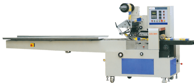
DZB300W Automatic Pillow Packing Machine 自动枕式包装机 Packing Capacity/包装速度: 50-200 bags/min. Bag Size/制袋尺寸: L40-140mm, W20-100mm, H5-35mm L100-300mm, W40-140mm, H20-70mm Max. Film Width/最大膜宽: 300mm
