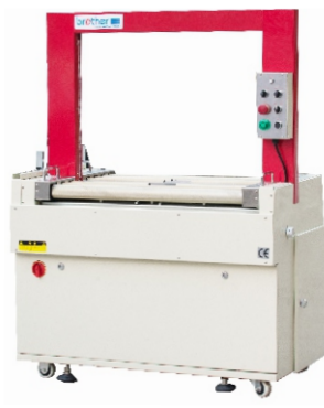
AP8060C (Online Model) Automatic Strapping Machine 在线式自动捆扎机 Power Supply/电源电压: 3P, 220V or 380V/50-60Hz Strapping Tension/捆扎力: 40-600N Adjustable Strapping Speed/捆扎速度: 2.18sec./cycle Strap Width/适用机用带宽度: 9-15mm Arch Size/框架尺寸: W800XH600mm
